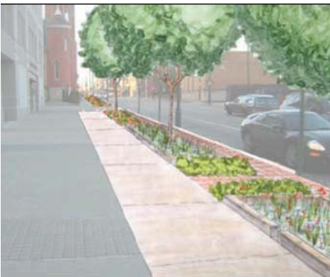
Photos (above): Creating a green street. The rendering shows how a major thoroughfare could be retrofitted to create stormwater management benefits, and a pedestrian buffer.
