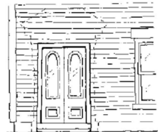
Removal of the door surround disrupts the historic proportion of the entrance. The door appears to be ungrounded, "floating" within the facade.
