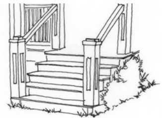
These simple railings are appropriate models for use with wooden porches.
